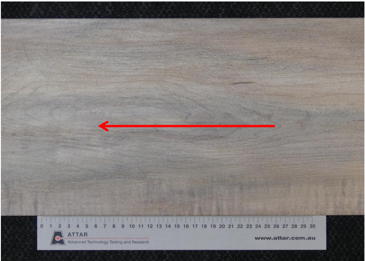
Figure 1: Aspecta 1 Bespoke 2.5mm / 0.7mm Wear Layer vinyl plank, Emboss: Natural Timber, Sample: Coventry Arrow indicates direction of testing
