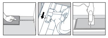
4. Starting second row: Rows can be started with end cuts if the cut plank is at least 30 cm long. If end cut is used for subsequent row a stair step pattern is established. Starting planks of random lengths will create a more aesthetic random stagger. Short end joints must not be closer than 20 cm to each other.
