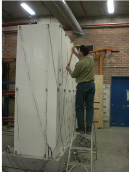
Fig 4.10 – Conducting Hammer Test on the specimen
