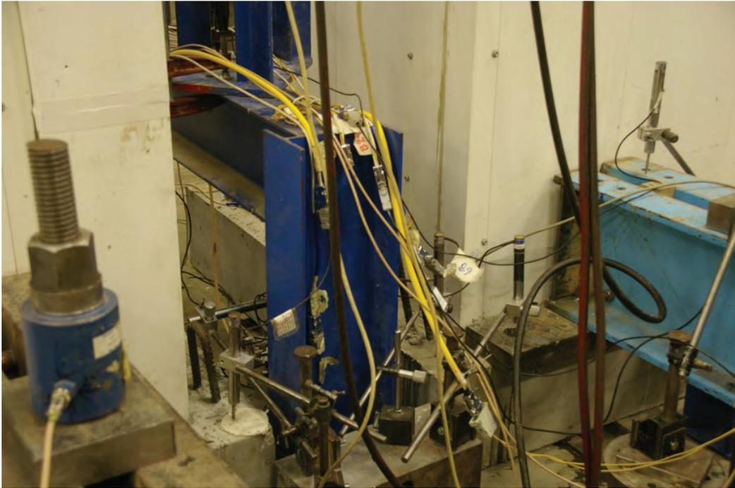
Figure 4.7 – bases of two Dincel walls on UTS strong floor ready for push over testing
