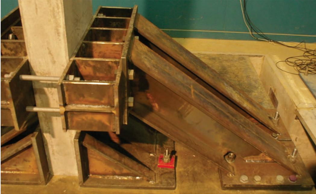
Fig 5.6 - Test set up (close up of the supporting structure)
