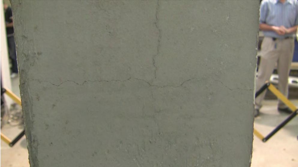
Figure 5.14 (e) Close Up View of Crack at X = 1150mm
