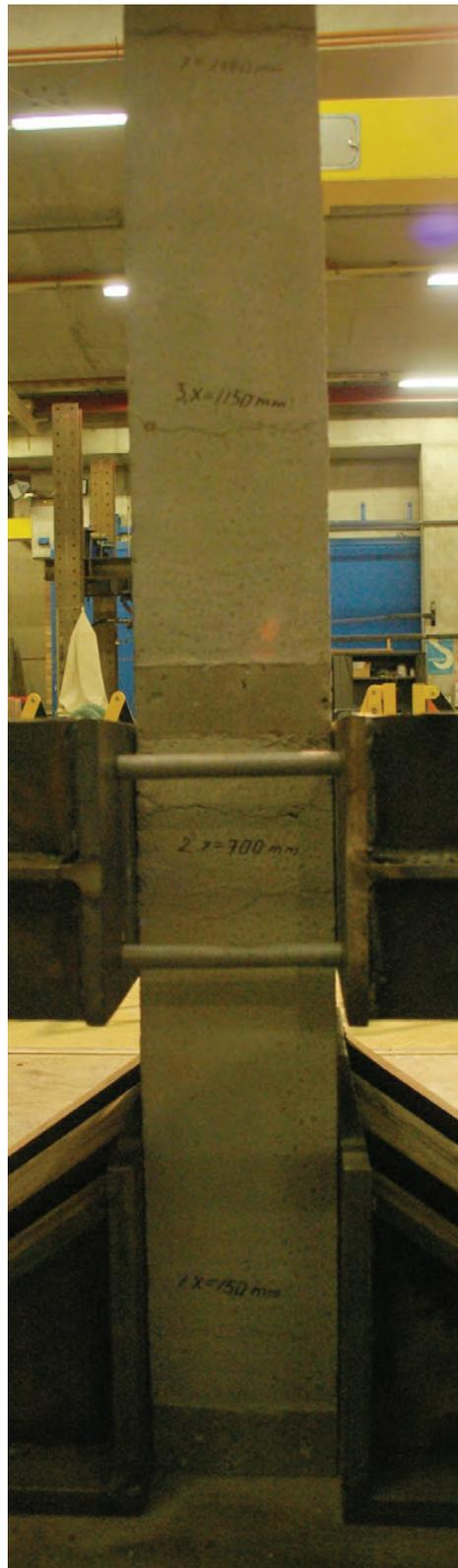
Fig 5.21 - Conventional wall at the conclusion of the tests
