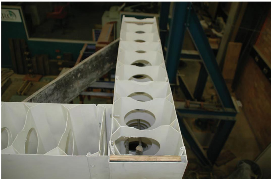
Fig 4.3 – Wall specimen ready for concrete pouring
