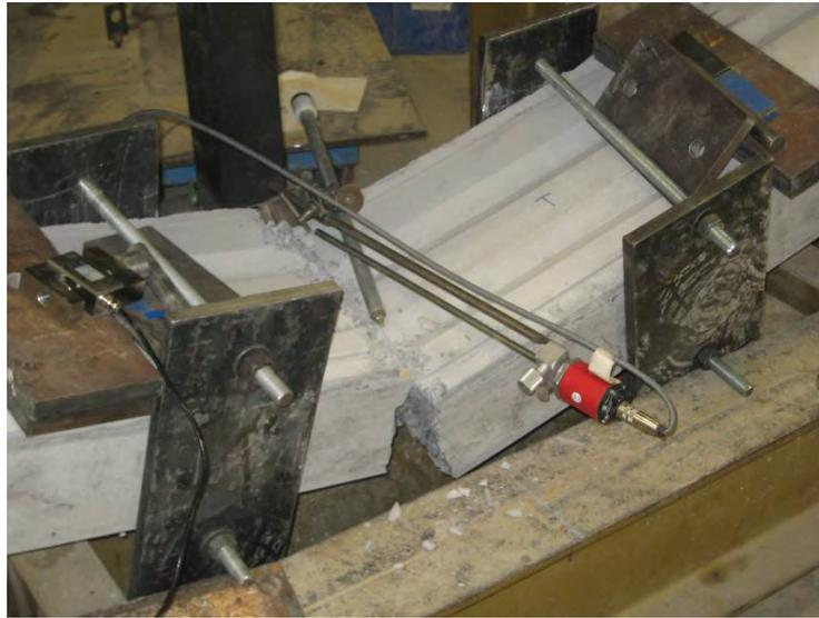
Fig 6.5 - Conventional Reinforced Concrete Beam Specimen after failure
