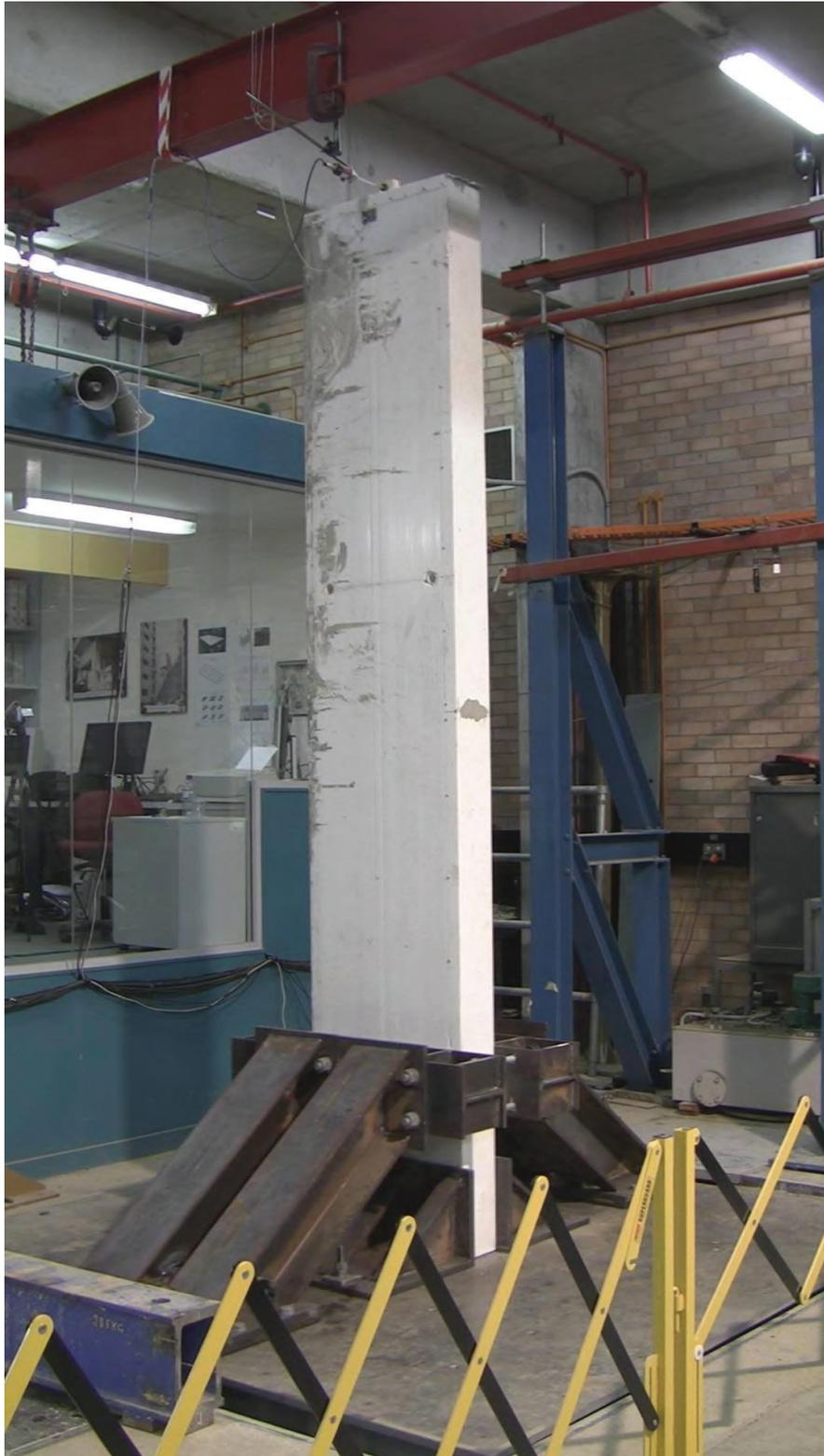
Fig 5.8 – Dincel System Sample 'C' set up on UTS Shake Table
