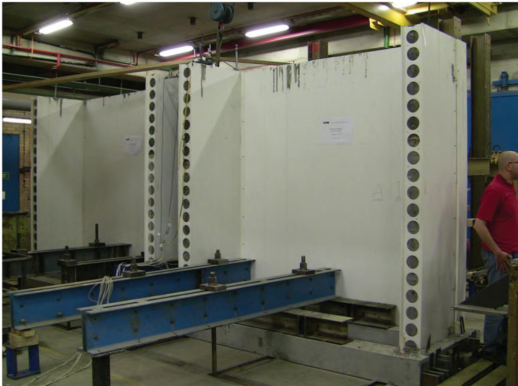
Figure 4.8 – Dincel Wall footing connection to strong floor
