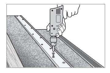
Once all screws are fastened, the profile installation is complete and the insert can be installed.
