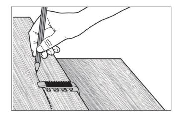
Step 4 Once carpet is installed, check the distance is correct using sample profile.
