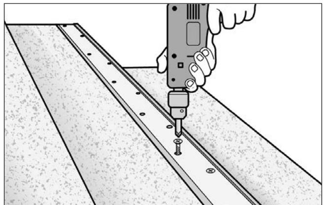
**Once all screws are fastened, the profile installation is complete and the insert can be installed.**
