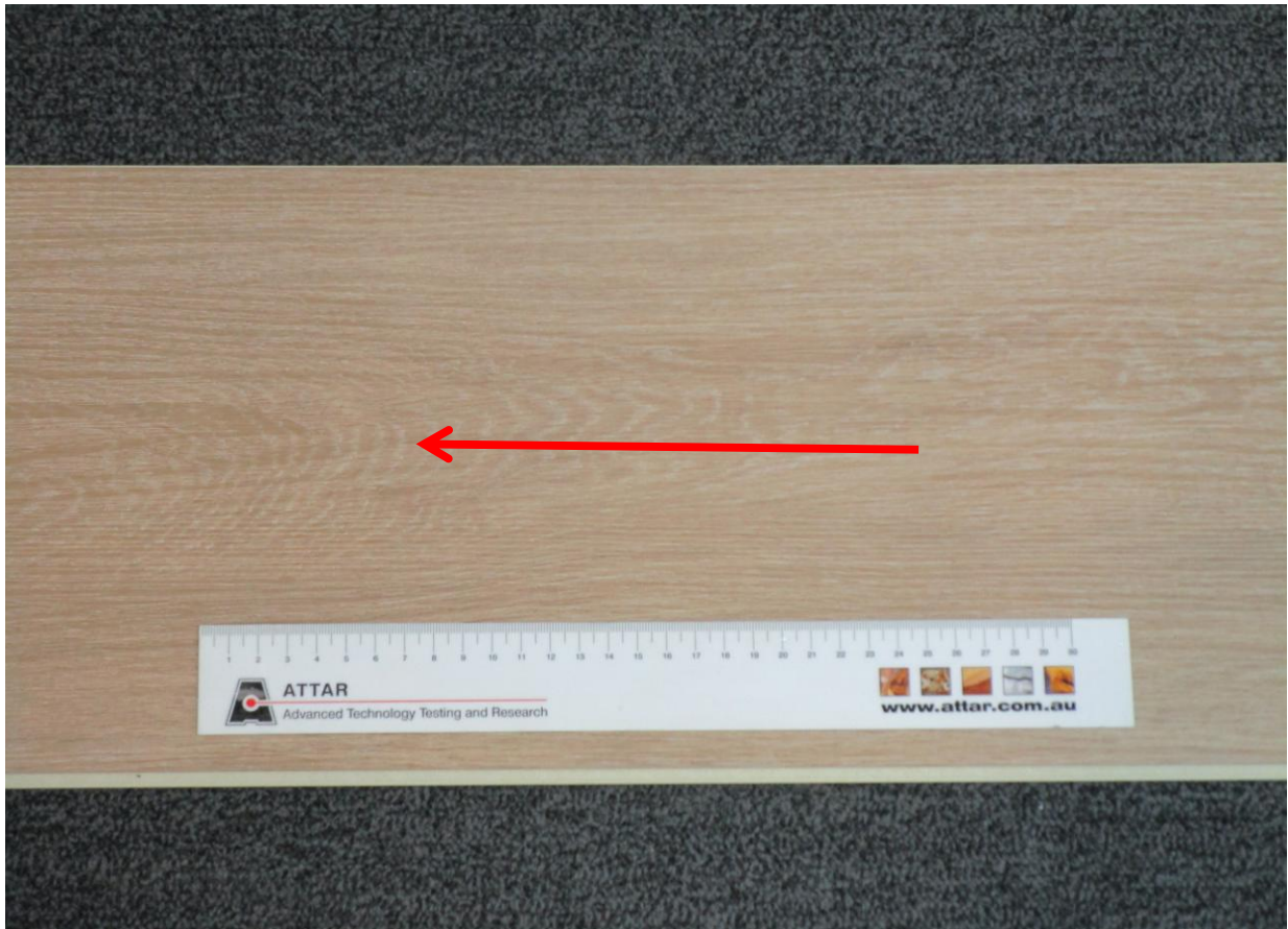
Figure 1: Korlok vinyl plank Arrow indicates direction of testing
