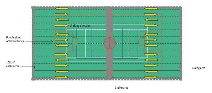
We recommend a dual-component epoxy glue, GreenLay Glue, reference Component A 1551057 Component B 1551058 – quantity to be applied, with a thin set of teeth spatula, between 300 and 350 gr per sqm. For a good installation you must carefully follow the manufacturer recommendations in particular, the waiting time before applying the covering. Then compact the surface with a roller to eliminate any bubbles that might remain between the sub-floor and the covering.
