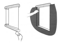
Alternative 2: At window-recesses the wall covering is rolled out over the window area and is then folded into the reveals. Loose pieces are inserted at the bottom recess, and at the top recess where necessary. The loose pieces are joined to the wall covering with welded seams.
