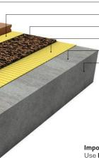
Approved engineered timber REGUPOL adhesive 40-203 (green) **REGUPOL** sonus eco 5 REGUPOL adhesive 40-203 (green) REGUPOL barrier 99-101 (white/yellow) Concrete slab prepared to AS1884
