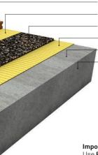
Approved engineered timber REGUPOL adhesive 40-203 (green) **REGUPOL** sonus multi 4.5 REGUPOL adhesive 40-203 (green) REGUPOL barrier 99-101 (white/yellow) Concrete slab prepared to AS1884
