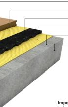
Approved engineered timber floor REGUPOL adhesive 40-203 (green) **REGUPOL** sonus curve 6 REGUPOL adhesive 40-203 (green) REGUPOL barrier 99-101 (white/yellow) Concrete slab prepared to AS1884
