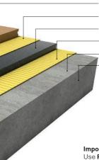
Approved engineered timber REGUPOL adhesive 40-203 (green) **REGUPOL** sonus core 10-S REGUPOL adhesive 40-203 (green) REGUPOL barrier 99-101 (white/yellow) Concrete slab prepared to AS1884
