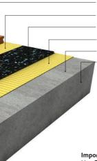
Approved engineered timber flooring REGUPOL adhesive 40-203 (green) **REGUPOL** sonus core 5 REGUPOL adhesive 40-203 (green) REGUPOL barrier 99-101 (white/yellow) Concrete slab prepared to AS1884
