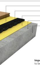
Approved engineered timber floor REGUPOL adhesive 40-203 (green) **REGUPOL** sonus curve 8 REGUPOL adhesive 40-203 (green) REGUPOL barrier 99-101 (white/yellow) Concrete slab prepared to AS1884
