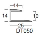
In this example, DT050 has been used with an LVT floor covering. The profile allows for a clean finish between wall and flooring and covers the expansion gap between surfaces.
