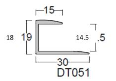
In this example, DT051 has been used with a wooden floor covering. The profile allows for a clean finish between sliding door and flooring and covers the expansion gap between surfaces.
