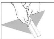
To glue the triangle-shaped piece more simply and securely, cut a groove on the back of the triangle with Tarkett Corner Knife. The depth of the groove shall be no deeper than half of the sheet thickness.
