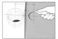
Around drain pipes, fold the sheet against the pipe and mark a line on the material where the center if the pipe is. Cut a hole about 25 mm (about 1 in.) smaller than the diameter of the pipe. As shown, cut the hole at the start of the fold. Heat the sheet vinyl and press it over the pipe. trim off excess material with o hook knife so that the break in the pipe wall is cleared.
