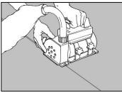
The sheets are hot welded. Do not weld until the adhesive has bonded completely, wait 24-48h. The joints are chamfered or grooved to about 3/4 of the thickness using a hand grooving tool or machine prior to welding.
