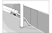
Around pipes by walls, cut the sheet and press it against the pipe to form a collar. In tight or cramped areas between pipes and walls, cut as shown by the dotted line. If a cover is required, do the following:
