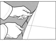
When the width of the room exceeds the sheet width (more than one piece has to be installed to cover the area), mark a line on the floor parallel to the longitudinal wall at a distance equivalent to 12 cm (about 41/2 in.) less than the sheet width. Mark the room's center on this line. On the bottom of each sheet, mark their center. The cross marks on the subfloor and sheets shall coincide at installation.
