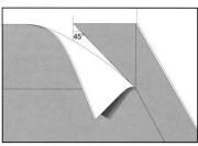
The corner seam shall be placed on one of the walls at a 45-degree angle.
