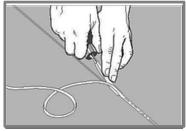
Trim with the chamfering-knife for Granit Multisafe/Optima Multisafe or equivalent. If the raised studs of the embossed pattern are too close to the seam area, cut them off before trimming of the welding thread.
