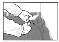
When fitting in-corners, make a cut in the excess material starting about 5 mm (about ½ in.) above the floor in the corner. If the material has to be heated before folding, heat the area between the sheet and the wall. This provides better contact between the sheet and adhesive.
