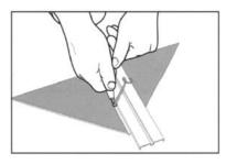
To glue the triangle-shaped piece more simply and securely, cut a groove on the back of the triangle with Corner Knife. The depth of the groove shall be no deeper than half of the sheet thickness.
