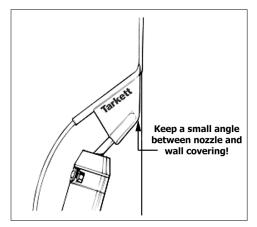
Remember to maintain a constant angle between the welding nozzle and the wall to preheat the joint properly.
