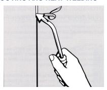
All seams are grooved using Tarkett Seam grooving Tool. Groove to about 3/4 of the thickness.
