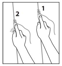
Welded seams must be allowed to cool to room temperature before they are trimmed. For best results, trim excess welding rod in two stages.
