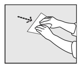
Press the sheet firmly using a piece of board with rounded edge or equivalent tool. Work from top down and from the middle to the sides of the sheet. IMPORTANT: Make sure you remove all trapped air.
