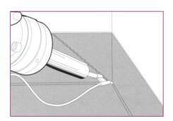
Use a hot-air gun for welding with thread at in-corners and out-corners. Tarkett Speed Welding Nozzle is specially designed for this purpose. For a perfect job, the Tarkett Swan Neck is required to effectively seal all seams nearest to the floor.
