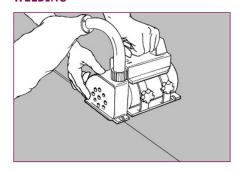
The sheets are heat welded. Do not weld until the adhesive has bonded completely. The joints are grooved to about <sup>3</sup>/<sub>4</sub> of the thickness.
