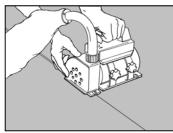
The sheets are heat welded. Do not weld until the adhesive has bonded completely. The joints are chamfered or grooved to about ¾ of the thickness using a hand grooving tool or machine prior to welding. Extra special care must be taken so that copper strips not are damaged during chamfering /grooving.
