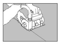
The sheets are hot welded. Do not weld until the adhesive has bonded completely, wait 24-48h. The joints are chamfered or grooved to about <sup>3</sup>/<sub>4</sub> of the thickness using a hand grooving tool or machine prior to welding.
