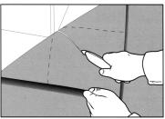
When fitting an out-corner, the sheet is folded against the corner and cut about 5 mm( ¼ in.) from the floor. The guidelines in the picture show the corner on the sheet and the position of the cut at about a 45degree angle. Then a diagonal cut is made as shown.
