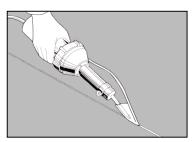
Weld with hot-air and Tarkett Speed Welding Nozzle. Carry out a test welding on a leftover piece before commencing work, to adjust speed and temperature **IMPORTANT:** When welding iQ Megalit, a Tarkett Speed Welding Nozzle or equivalent should be used.
