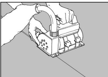
The sheets are hot welded. Do not weld until the adhesive has bonded completely, wait 24-48h. The joints are chamfered or grooved to about ¾ of the thickness using a hand grooving tool or machine prior to welding.
