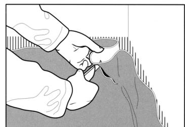
When fitting in-corners, make a cut in the excess material starting about 5 mm (about 1/4 in.) above the floor in the corner. If the material has to be heated before folding, heat the area between the sheet and the wall. This provides better contact between the sheet and adhesive.
