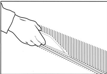
Using a straight edge and pencil, mark at a height of about 10 cm (approx. 4 in.) all walls where the flooring will be covered. Apply the adhesive on the walls up to the marked line, using a fine-notched trowel. Spread some of the adhesive out onto the floor, as shown in the picture.
