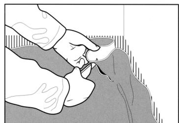
When fitting in-corners, make a cut in the excess material starting about 5 mm (about 1/4 in.) above the floor in the corner. If the material has to be heated before folding, heat the area between the sheet and the wall. This provides better contact between the sheet and adhesive.
