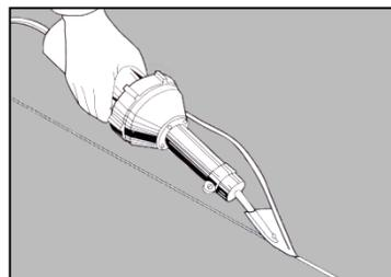
Weld with hot-air and Tarkett Speed Welding Nozzle. Carry out a test welding on a left-over piece before commencing work, to adjust speed and temperature **IMPORTANT:** When welding iQ Megalit, a Tarkett Speed Welding Nozzle or equivalent should be used.
