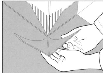
The triangle can now be folded and placed on the corner. It will overlap the covered floor. Cut through the overlapping material to make a tight fit.
